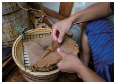
9. A wooden roller is used to firmly press the water out of the paper, which is then sandwiched between rush mats in stacks of several sheets to further remove the moisture. This step is called *nureposhi* (“drying”).
