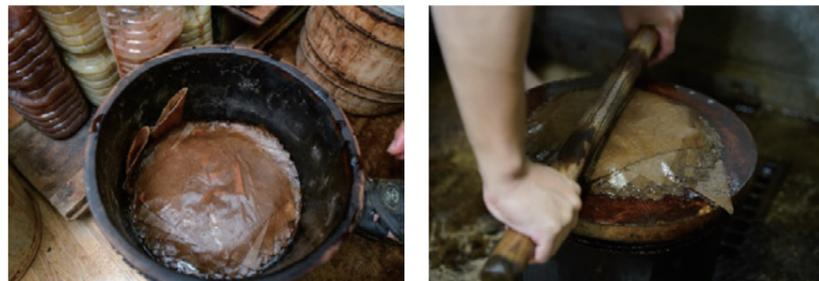
10. The sheets are peeled apart and bundles of multiple sheets are beaten with the mechanized hammer to evenly distribute the moisture (*aku-uchi*).
